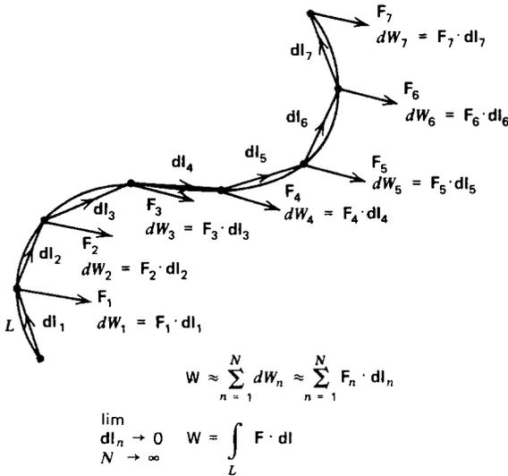
Figure 1-11 The total work in moving a body over a path is approximately equal to the sum of incremental works in moving the body each small incremental distance  $d\mathbf{l}$ . As the differential distances approach zero length, the summation becomes a line integral and the result is exact.
