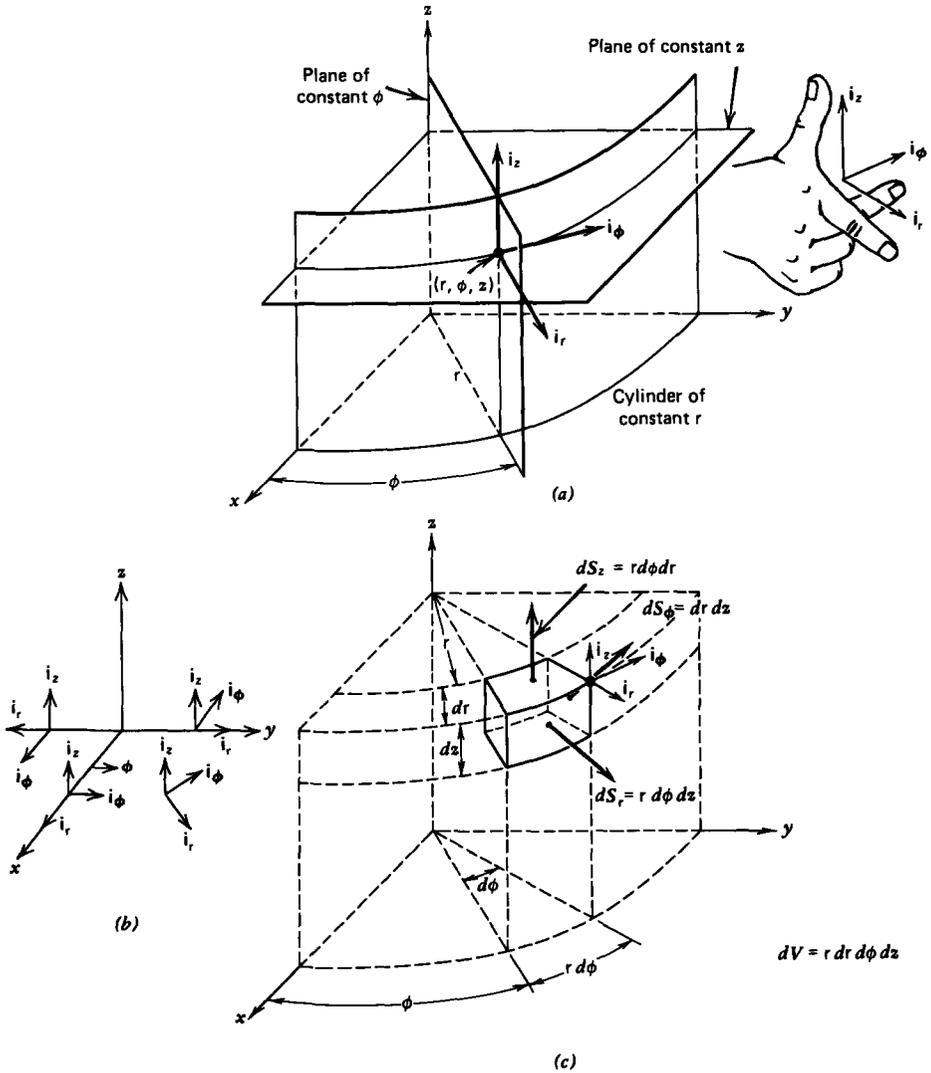
Figure 1-2 Circular cylindrical coordinate system. (a) Intersection of planes of constant  $z$  and  $\phi$  with a cylinder of constant radius  $r$  defines the coordinates  $(r, \phi, z)$ . (b) The direction of the unit vectors  $i_r$  and  $i_\phi$  vary with the angle  $\phi$ . (c) Differential volume and surface area elements.
