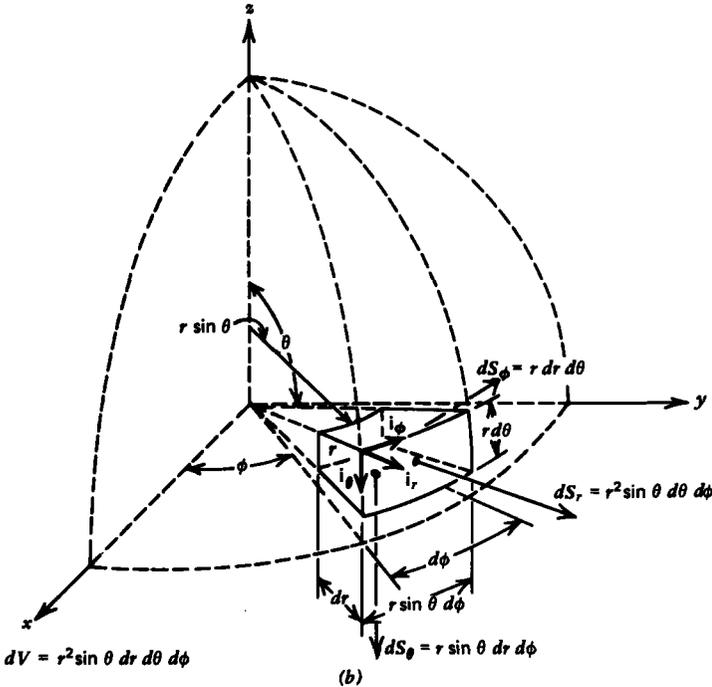
Figure 1-3 Spherical coordinate system. (a) Intersection of plane of constant angle  $\phi$  with cone of constant angle  $\theta$  and sphere of constant radius  $r$  defines the coordinates  $(r, \theta, \phi)$ . (b) Differential volume and surface area elements.
