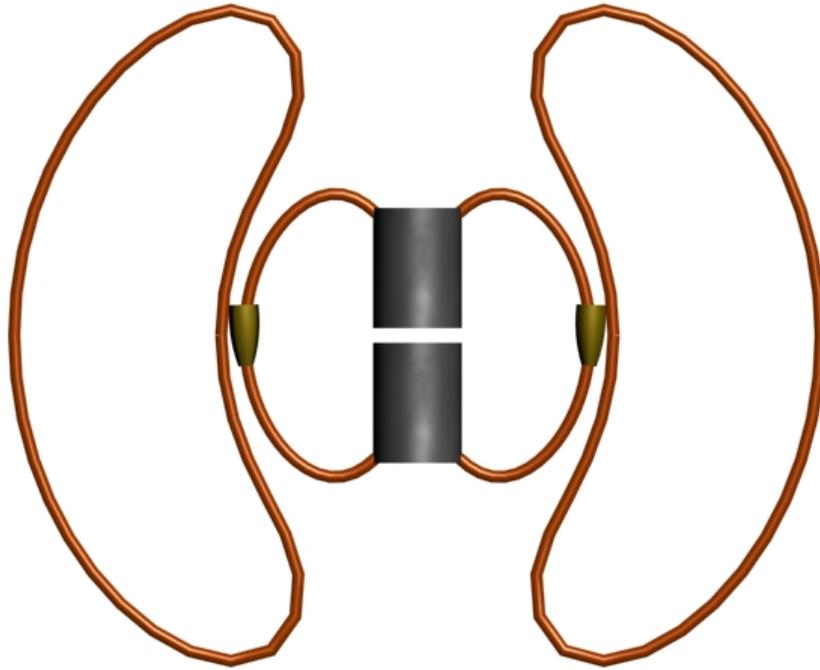
**Answer: (1) The current is about zero. The charge on the top half of the antenna is at its maximum value, and therefore the current, which is the time rate of change of the charge, must be near zero.**
