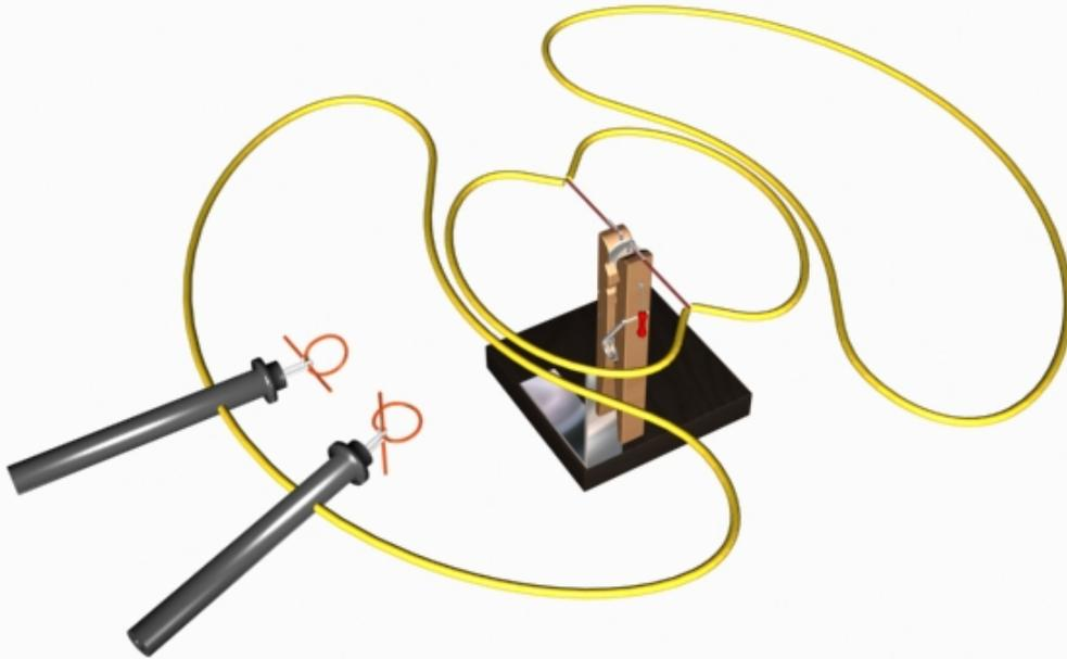
**Answer: 1. The electric field pattern from the spark gap antenna is shown above. When positioned as shown, the receiving antenna gets maximum power when parallel to the transmitting antenna wire, because the electric field can then drive the maximum current in the receiver. We say that the wave is “polarized” in the direction of the E field.**
