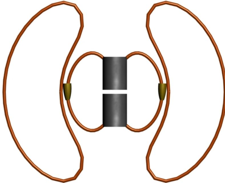
**At the time shown the charge on the top half of our  $\frac{1}{4}$  wave antenna is positive and at its maximum value. At this time:**
