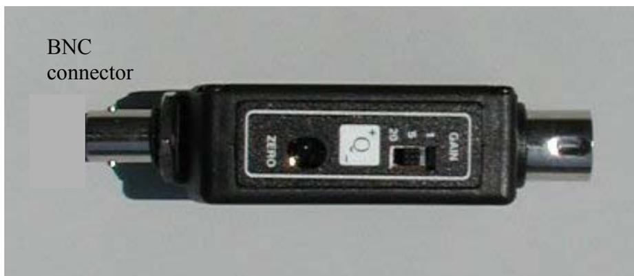
**Figure 5** Gain and Zero Settings for Charge Sensor.
