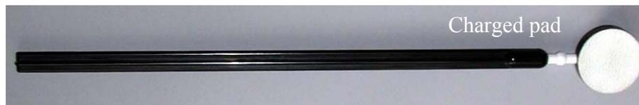
**Figure 3** Charge Producer
