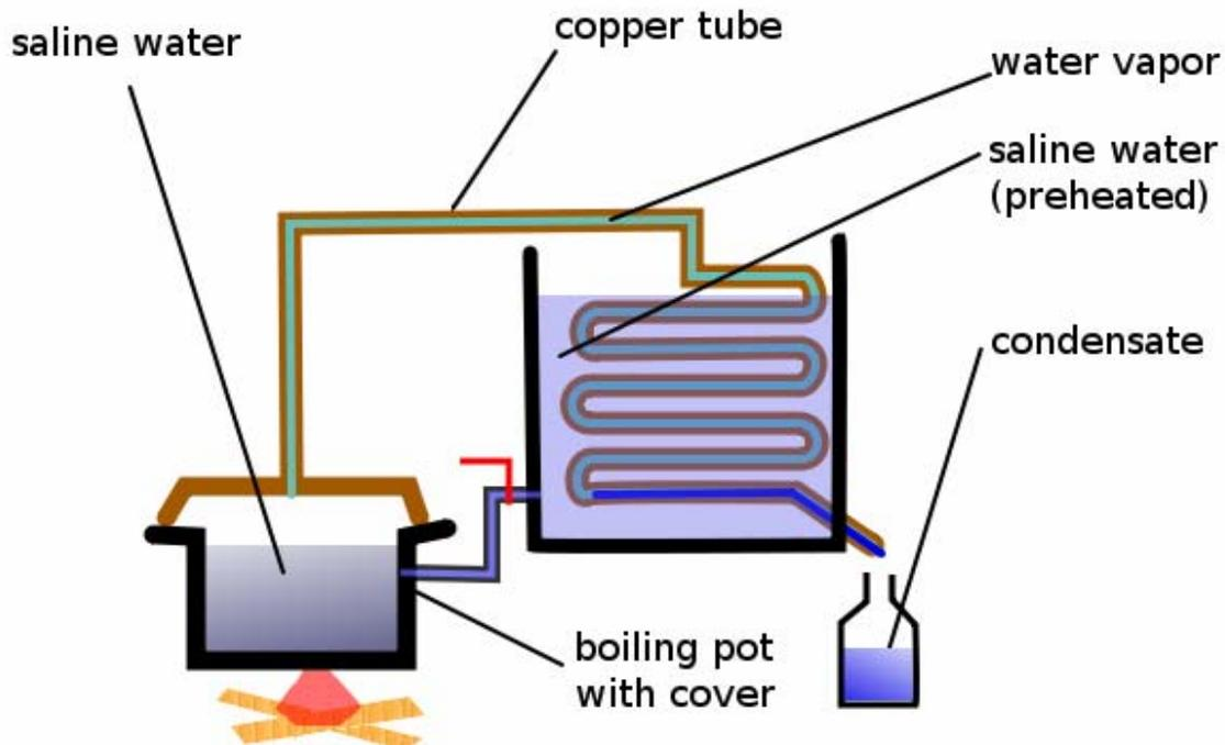
**Figure 3: Single Effect Evaporation System**
