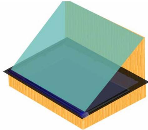
**Figure 4: Solar still made from wood and local material**
