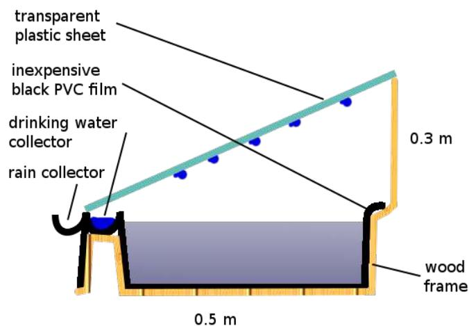
**Figure 5: Section view of a solar still**
