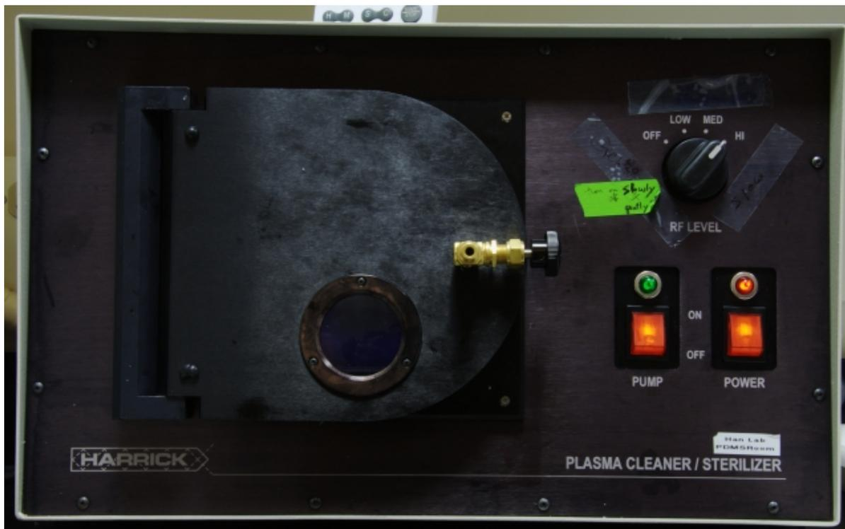
The vacuum pump has two indicators that tell you when the vacuum is ready. First, a light on the pump itself turns from yellow to green. Second, the vacuum gauge shows that the pressure drops to about 65 mbar (i.e., 65/1000 of atmospheric pressure) and stabilizes there. At this point you can turn the RF signal on to the highest setting. When you do so, you should see a purple glow coming from the inside of the chamber.
