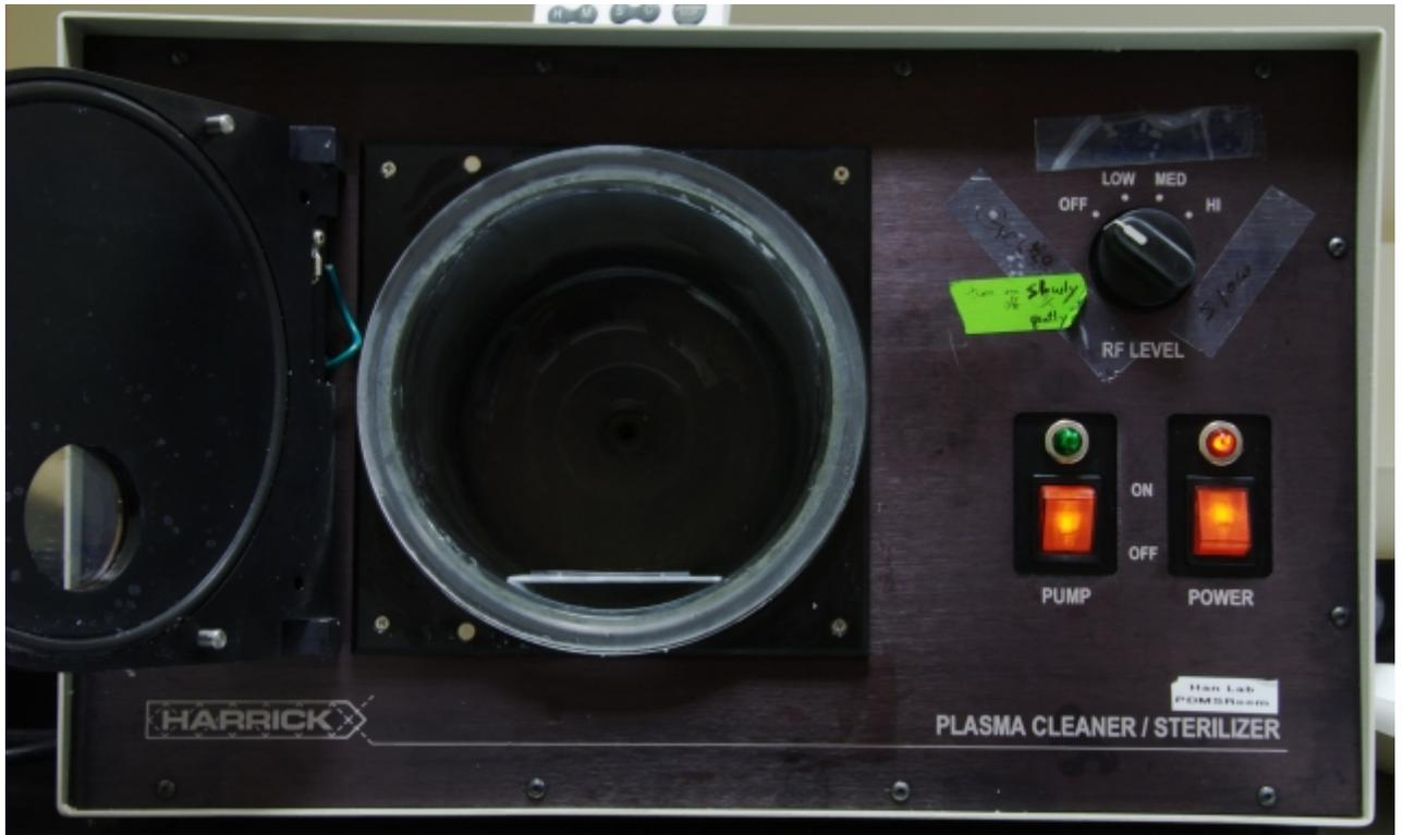
Close the chamber door, close the release valve (the picture below shows the device with the release valve closed; compare it to the first picture above). Flip both switches to the "On" position, but do not turn up the RF level yet.
