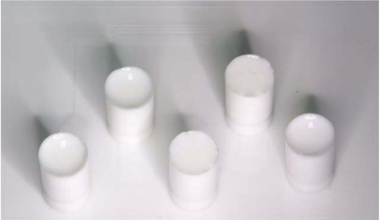
A third technique is to cast reservoirs out of PDMS. This technique has all of the advantages of the cylinder method, and can be tapered at the bottom to prevent clogging. It has the disadvantage of requiring another casting and bonding step. First, tapered cylinders like the one shown below are cast to form a mold.
