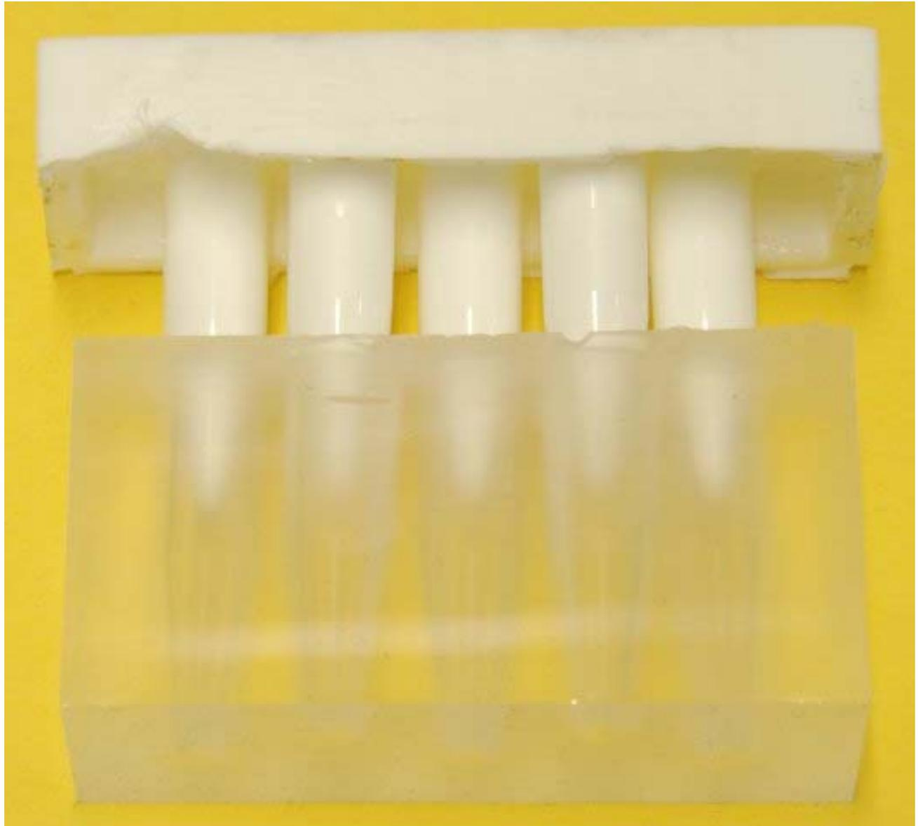
Since the bottom surface will be bonded to a PDMS device, it must be smooth. To ensure smoothness, a glass chamber is built out of microscope slides to surround the plastic mold. PDMS is then poured into this chamber to cast the reservoirs. The resulting reservoirs have smooth, optically clear surfaces.
