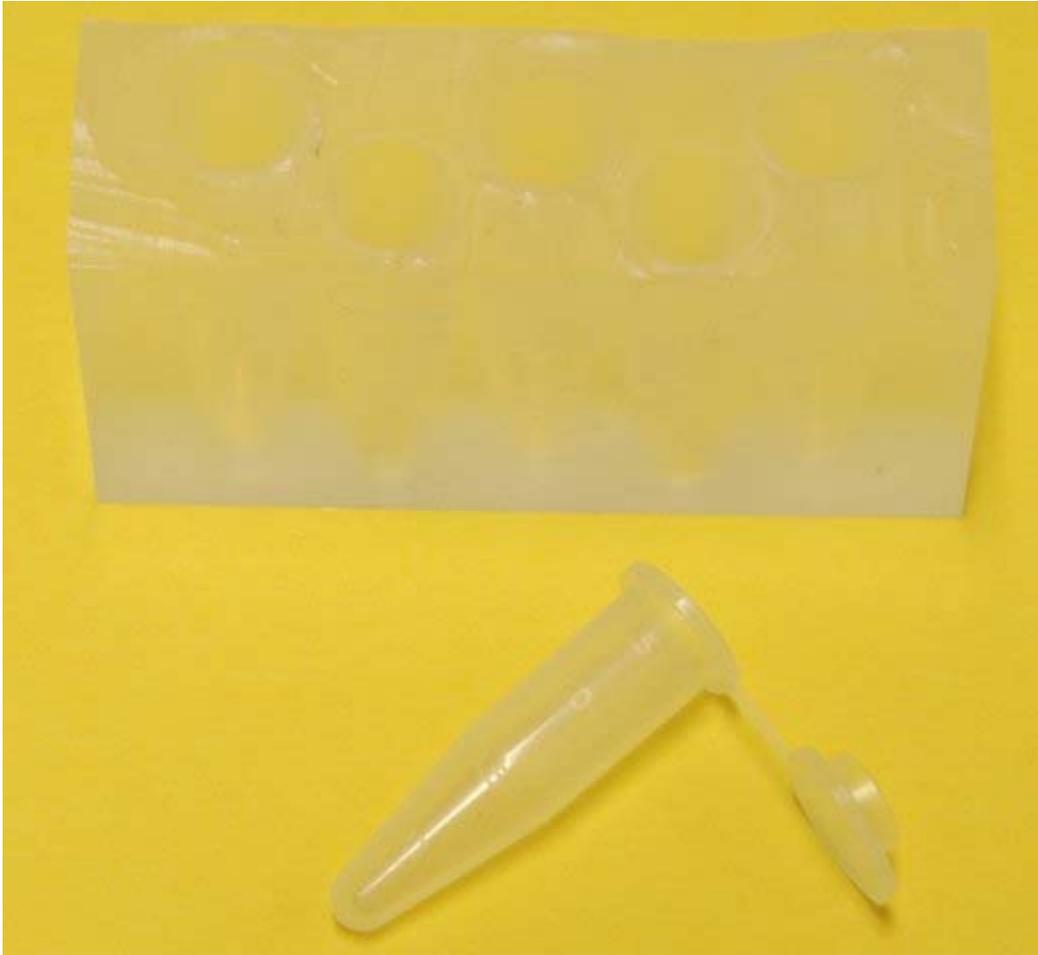
This mold is then used to create a plastic negative. The plastic negative is used to cast the reservoirs in PDMS.
