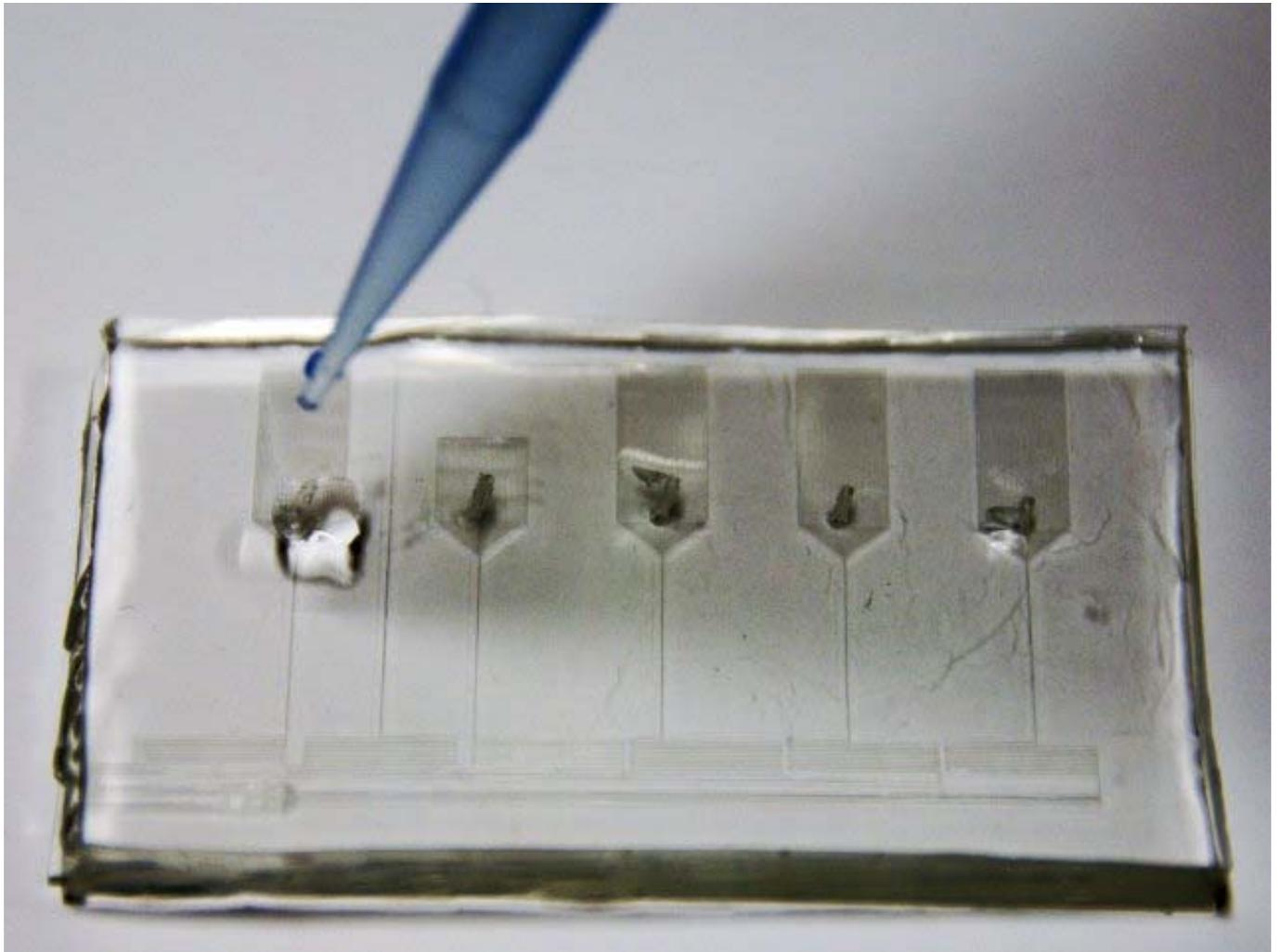
Next, a pipette tip filled with fluid is inserted into the hole. The pipette tip must not contain any air bubbles. One advantage of this technique is simplicity; it is relatively easy
