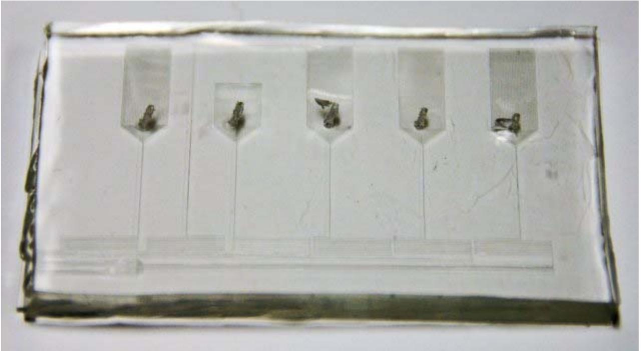
First, we place a small droplet of deionized (DI) water over the hole. This ensures that when we insert the fluid-filled pipette tip, we do not push air into the channel.
