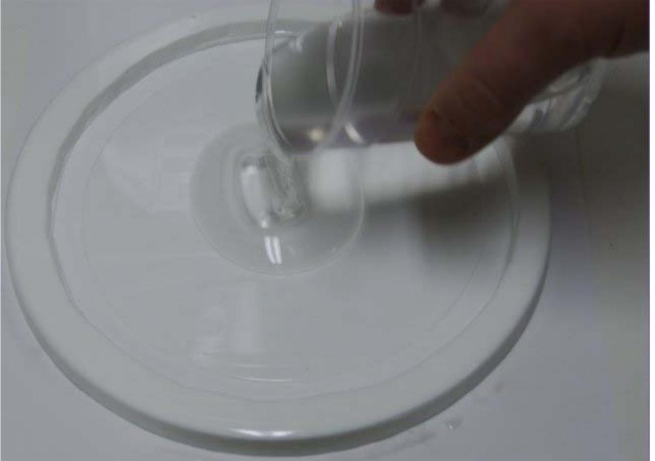
When you are done pouring, the entire device should be covered in PDMS, as shown below.
