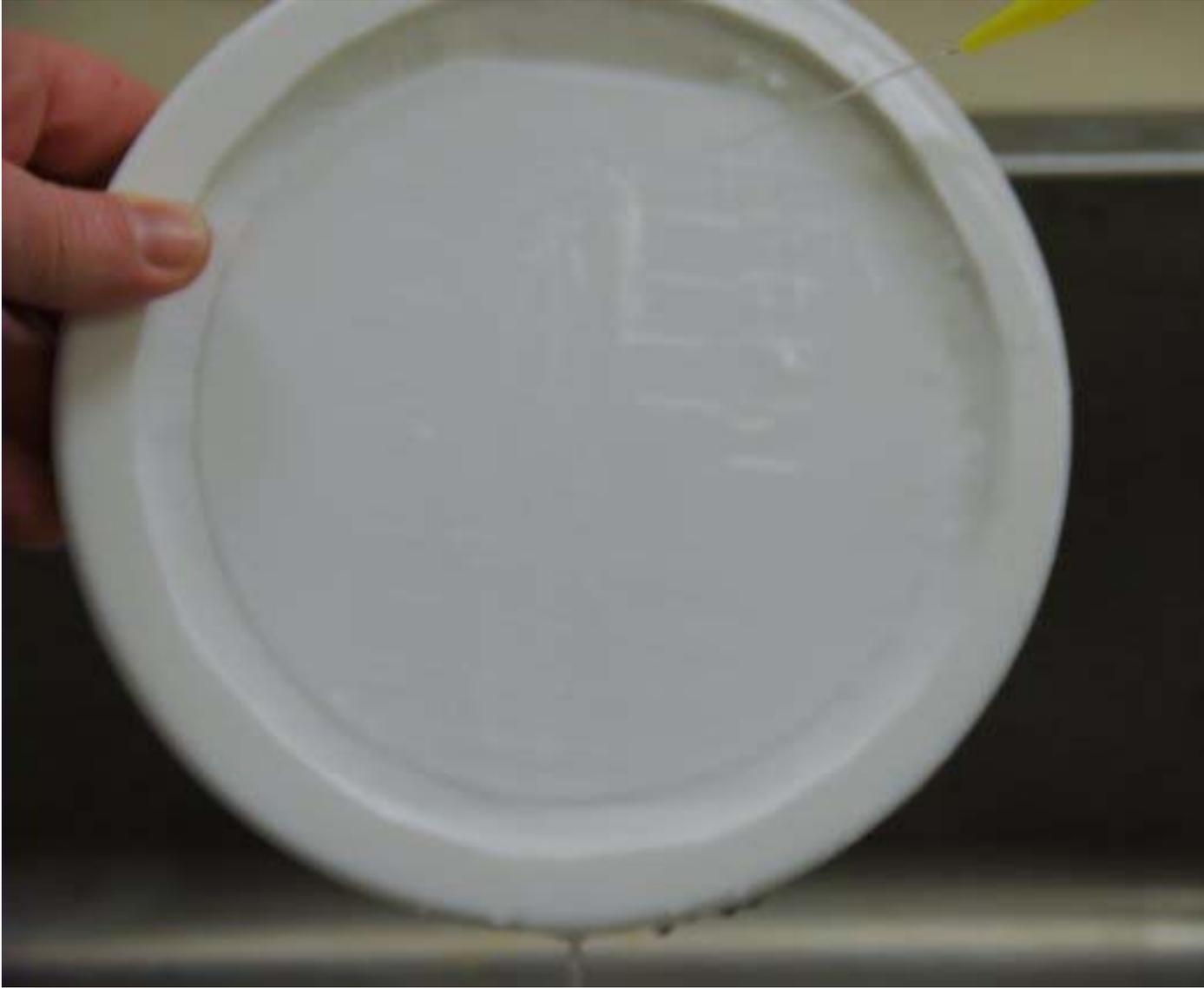
The master should then quickly be dried with pressurized air, either from an air canister as shown here or from a central air pump.
