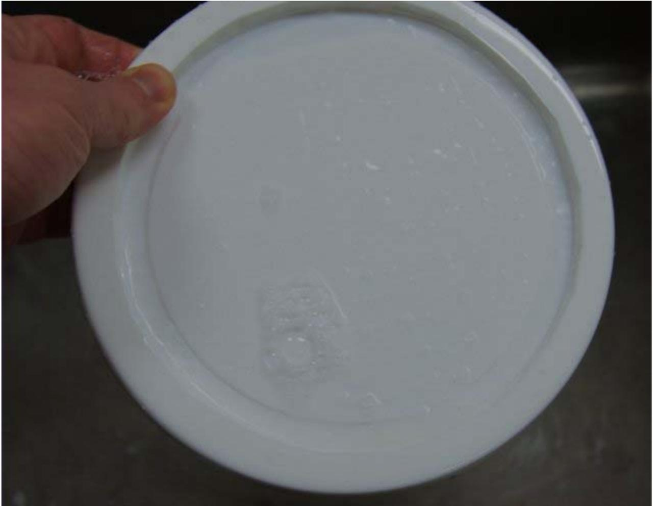
After washing the master, it should go through several rinse stages. First, rinse it with deionized (DI) water. This removes residue left behind by the tap water.
