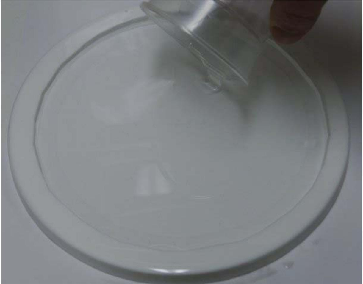
After the PDMS is poured, carefully place the master into the oven. Be careful not to spill any PDMS while you are moving the master! The image below shows what you should **NOT** do: do not place the master directly on the cooking rack! Instead, place it in a secondary container, such as a teflon pan. That way, any PDMS that spills out of the master will be caught by the pan.
