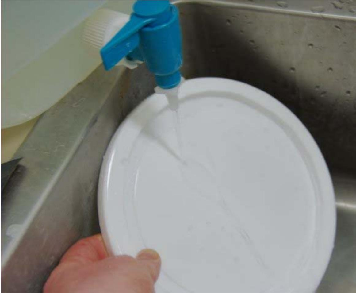
Next, it should be rinsed with isopropyl alcohol. This step picks up oils and other debris that can affect the casting.
