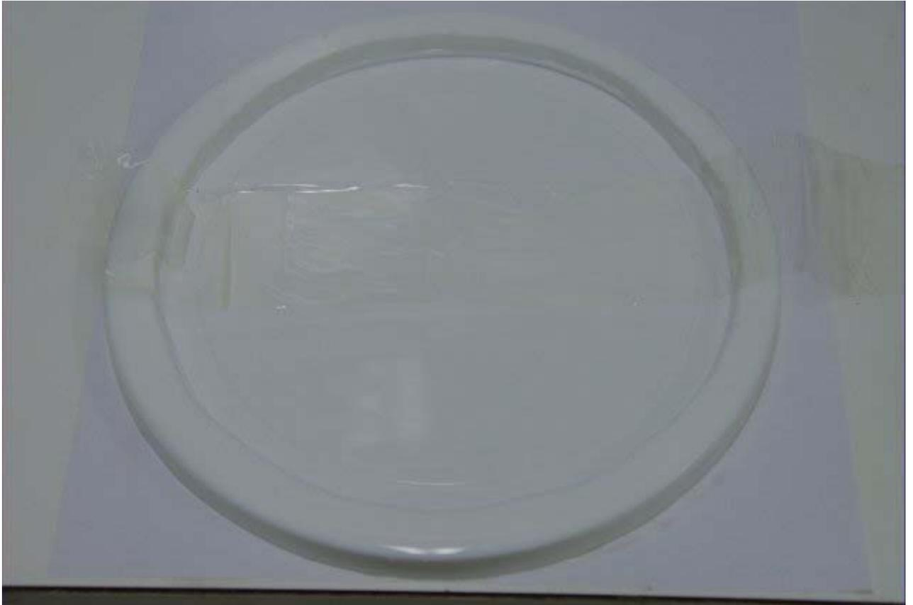
When pouring PDMS, it is important to try to minimize the formation of air bubbles. If you have too many air bubbles, you may need to de-gas the master before baking the PDMS. One way to minimize the formation of air bubbles is to pour the PDMS as close to the master as possible. The image below shows an example of how to pour. The PDMS should flow out of the cup onto the device, rather than drop.
