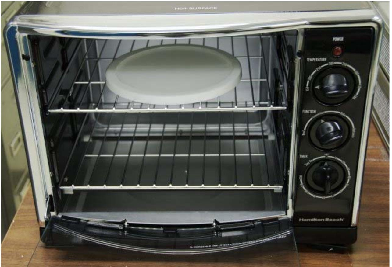
The PDMS needs to bake for at least an hour before it is hardened. Preferably it should bake for two hours or more. The oven should be set to 150 degrees F, on convection mode. The image below shows the proper oven settings for a one-hour bake.
