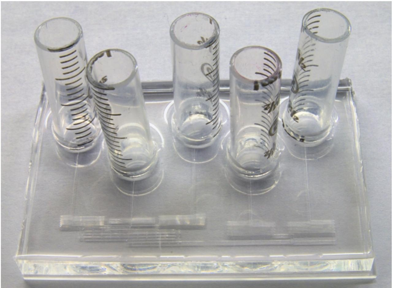
Rather than bonding the device to a glass slide as shown in the above image, though, the device is placed in the bottom of a plastic tray channel-side up. A quick-hardening plastic is poured over the device and allowed to solidify. The plastic takes the complementary shape to the device; that is, it becomes a new master. The plastic can easily be separated
