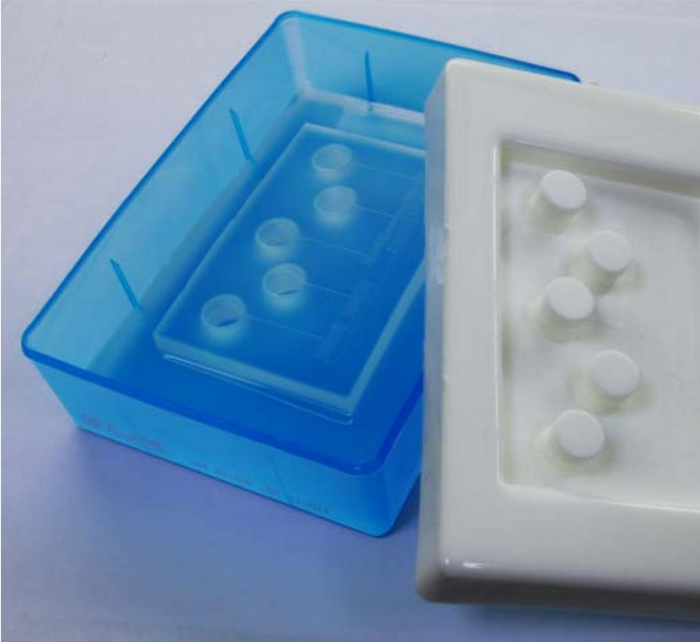
The resulting master is sturdy, can be used many times without loss of resolution, and can easily be modified. The images below show two variations of a single design, one which creates holes for inserting plastic cylinders and one which does not.
