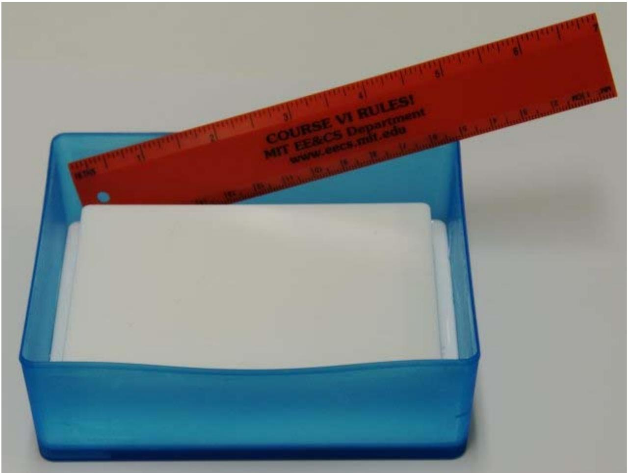
This mold is then used to create a PDMS container, such as the one shown below. The plastic mold can be saved and used to make a large number of PDMS casts.
