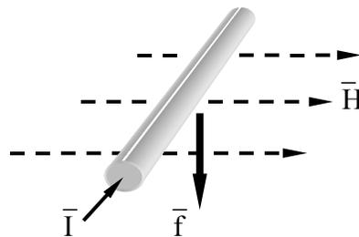
Figure 5.2.2 Magnetic force on a current-carrying wire.
