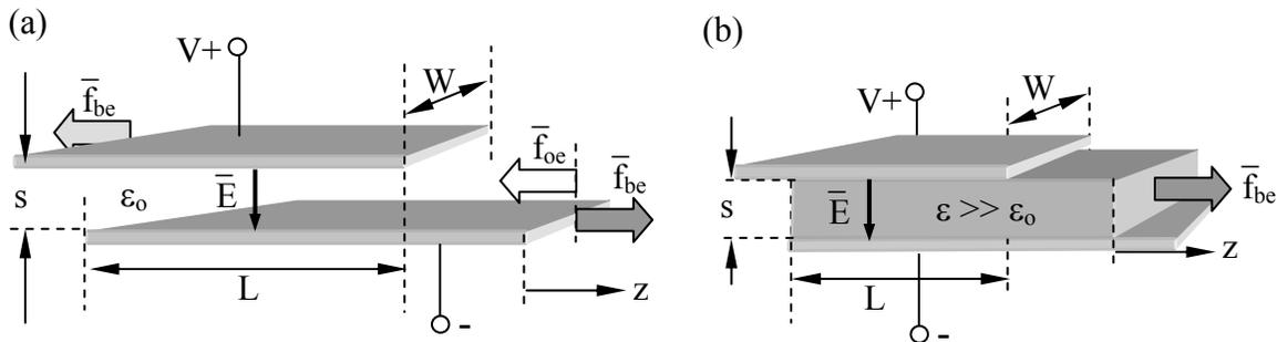
Figure 5.4.1 Capacitor plates and dielectrics being separated laterally.
